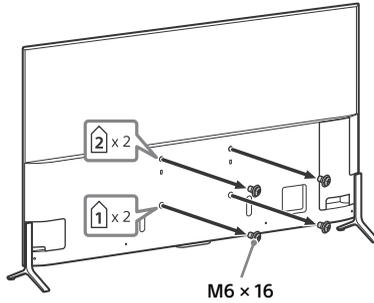
**3** Attach the U-shaped Bar ❶ (supplied with the TV) to the rear of the TV.
