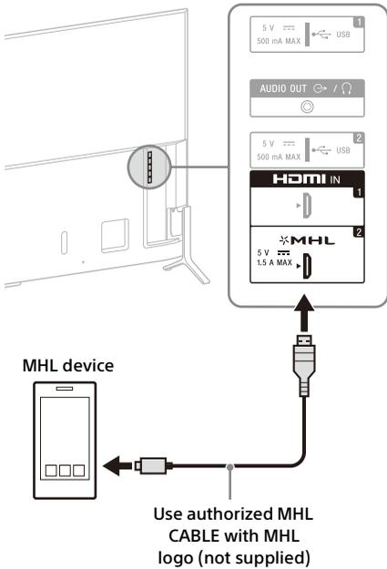
The TV simultaneously charges the MHL-compatible connected device while playing photo/music/video files. You can use the TV remote control to control the connected MHL-compatible device.
