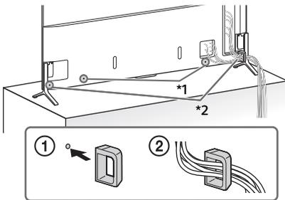
\*1 Location of cable clamer when the Table-Top Stand is attached to middle position.
