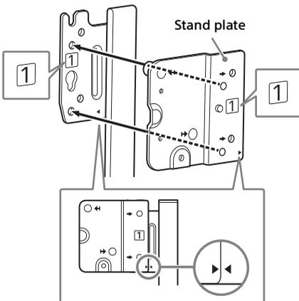
3 Fix the stand plate to the Table-Top Stand with screws (M5x10) (supplied with the TV).
