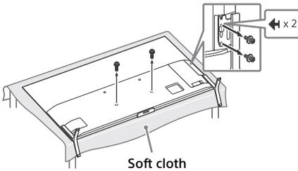
2 Attach the stand plate (supplied with the TV) to the detached Table-Top Stand.
