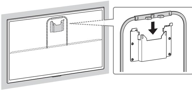
**12** Attach the lock plate (H1) (supplied with the TV).
